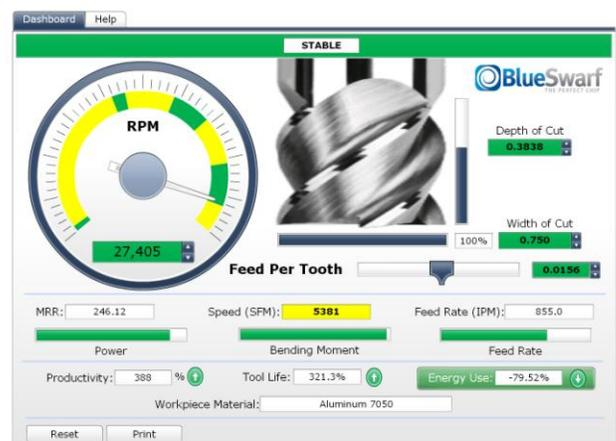
On the "RPM" dial of the Tool Dashboard, green zones represent the stable cutting areas for this particular tool. The Tool Dashboard makes it easy for the programmer to manipulate speed, depths of cut and chip load, and predict the effects of these changes based on the dynamics of the machine.
