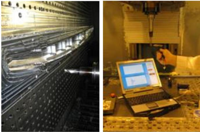
The tap test can find the spindle speed and depth of cut that will maximize metal removal rate for a particular combination of machining center, toolholder and milling tool.
