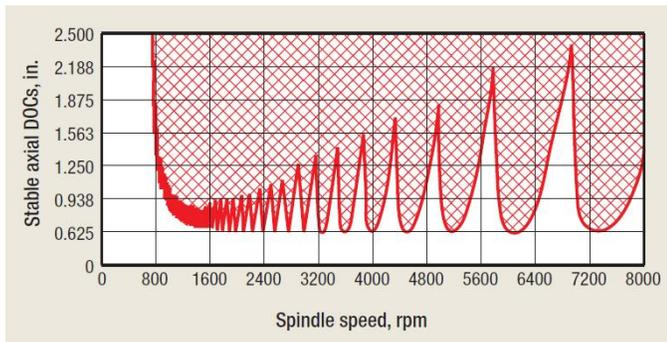
This example of a stability diagram shows the increased depths of cut that are possible within specific, narrow bands of spindle speed across the entire speed ranges. Tap testing is aimed at finding these stable speeds.
